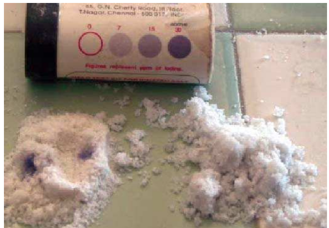
Unevenly iodized salt. The dark grey patch in the salt (left) indicates optimal iodate level. The light salt on the right was not sprayed with potassium iodate.
