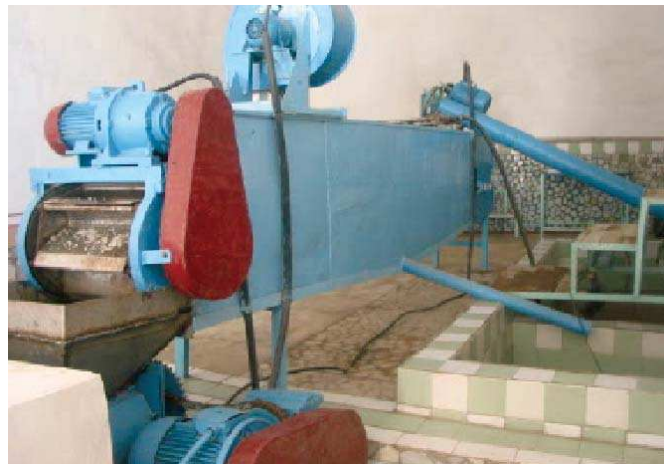
A salt iodizing machine.
