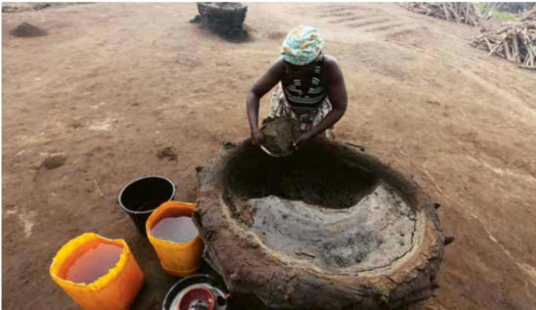
Small scale salt production in Djegbadji, Benin. Artisanal salt farmers here dig off the top layer of soil near their homes then filter water through the dirt to draw out salt. They later boil the water to collect the salt. ©Sunday Alamba.
